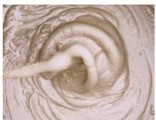
Manual application can be done in 1 or 2 coats, 10 to 20 mm thick.
