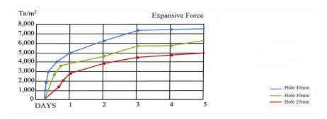
The expansive force of Topeca Dinamit increases progressively over the course of the day. For most materials sufficient to achieve 3. 000 Ton/m<sup>2</sup>.
