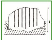
Example of extraction of stone / rock: hole  $\emptyset$  40mm, drilling 60 ° slope or less, consumption Topeca Dinamit =  $42kg/m^3$ .
