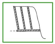
Concrete: hole  $\emptyset$  40mm, with main reinforcement and drilling previously sectioned parallel to the free face, consumption Topeca Dinamit =  $5 \text{kg/m}^3$ .
