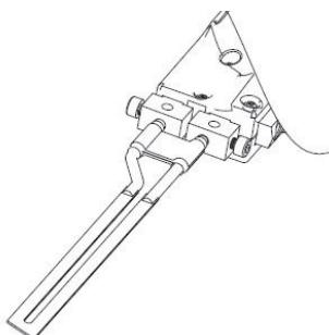
1. Loosen the screws on the blade holders with the wrench.
