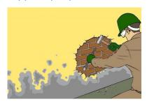
Degraded, loose plaster with a high salt load should be removed by chipping up to 50 cm above the visible damp part.
