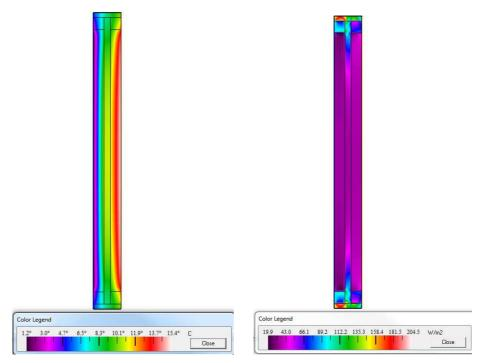
Figure 1: Distribution of temperature and heat flow with their related scales.
