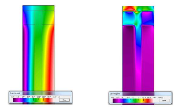
The next figure shows the distribution of temperature and heat flow in detail.
