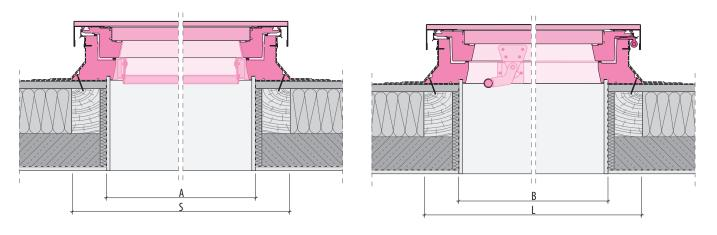
Special size DRL 27½" x 59½" with R.O. 27½" x 5" to create a step on a roof surface
